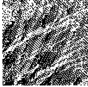
FIG. 1. A snapshot of the simulation. The system size is 100 \times 100 and p = 0.4 . The black and gray dots show right-directed and up-directed cars, respectively. There are some local jam clusters. Jam clusters are sorted out with the maximum throughput ( \rho = 2/3 ).
